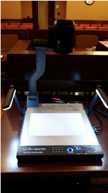
A Document cameras is available in each courtroom. The camera allows content to be presented through the video monitors. Objects are displayed on the witness monitor, judges monitor, podium monitor and attorney table monitors. Any object can be displayed including 3-D objects, negatives, photos, x-rays.
